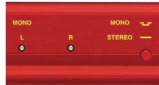
Fig 1-7: RB-DA6R Front Panel Input Gain Controls and Stereo/Mono Switch.
