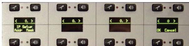
Figure 4-1: IC.20 Front Panel IP Address Displays BootP Server
