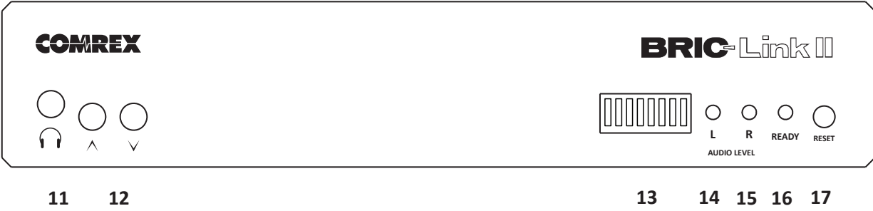
FIGURE 2 FRONT PANEL DIAGRAM AND DESCRIPTIONS
