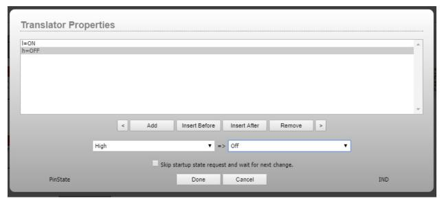
What we have just defined is that if the start point (GPI) is low, then we are going to set the LCD Button indicator on the button to On. If the GPI is high, then we are going to set the LCD button indicator to Off. We are essentially defining a list of rules as to what the endpoint should be depending on what the start point currently is.
