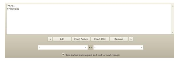
Without this option a restart of the system will request the current GPI state which is high and will therefore toggle the previous route. In many cases this will route nothing to the air chain because no previous state exists yet.
