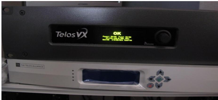
If you don’t see “The big OK”, there is an indication on the front panel and web GUI (system page) that will indicate what’s wrong. It’s usually a power supply not plugged powered, an ethernet not plugged in or the switch not set up for Livewire.
