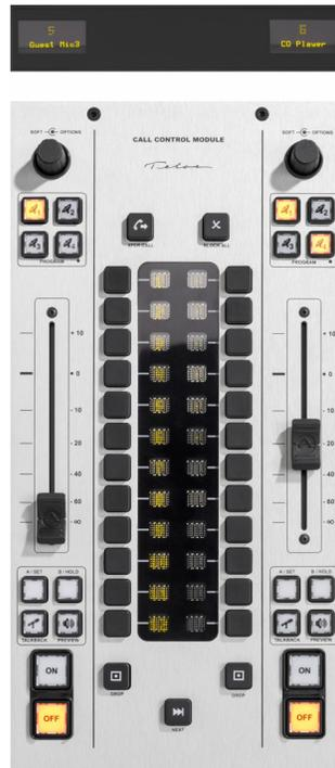
Integrating phone line selectors into the studio mixing console is an operator-pleasing feature that is easy to accomplish in a networked studio. As this is written in December 2017, the following consoles have VX-compatible call control modules available.
