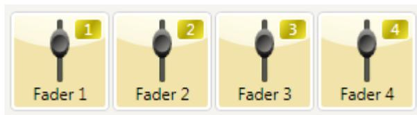
In older on-air phone systems, we were limited to one or two hybrids (audio paths), so we only used one or two console faders. With the VX system, this limitation is removed. That means that you can assign a fader to each call if you want to do so, allowing independent control of each call's volume.
