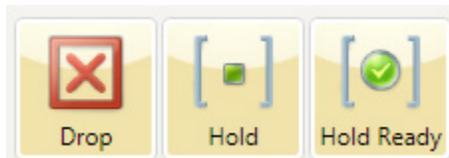
**Drop** disconnects a call that is ringing, active on the handset, or on-air. If more than one line is in this category, they will all be highlighted. Press the line that you want to drop. Or select the line you want to drop to highlight it and then press **Drop**.
