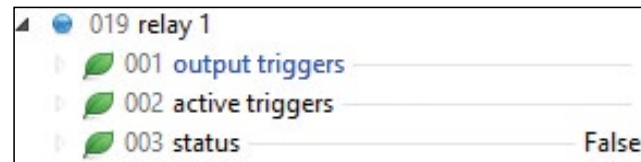
Fig 10-11: Ember+ Relay Branch Structure
