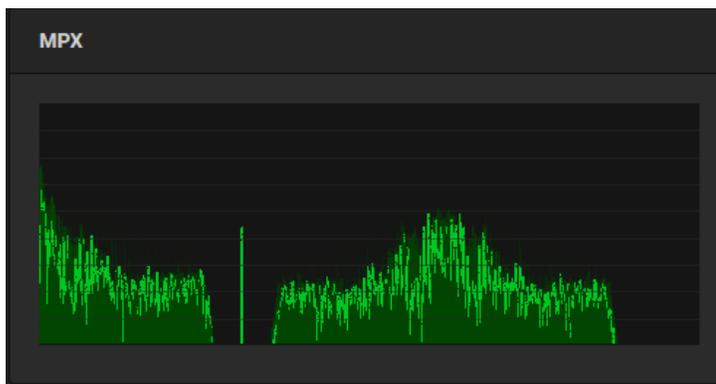
The MPX display provides a view of the FM signal, including L+R, 19kHz stereo pilot L-R, and RDS signals.
