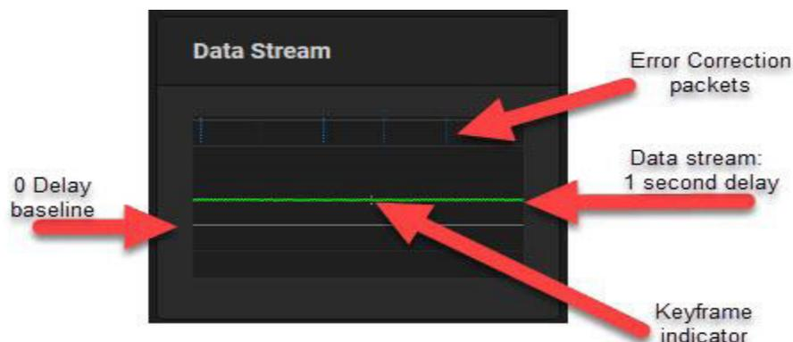
As you experiment with error correction settings in your Encoder, you can use the dashboard of your Decoder to observe cause and effect.
