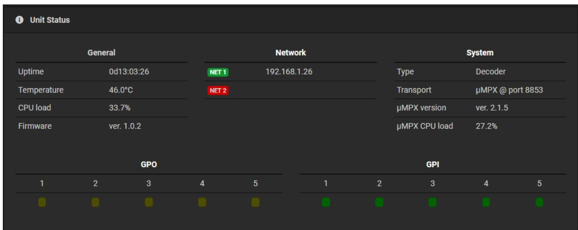
The Unit Status section of the Decoder Dashboard page provides general configuration, system and network information, and can be useful for checking the status of your unit for details like, uptime, CPU temperature and load and firmware versions.
