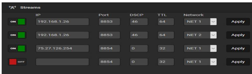
If you want to send more streams from your Encoder, you will need an extended license. Encoders can push up to 16 Unicast streams. Please note that the more Unicast streams you send, the more network uplink bandwidth is required, so be certain to factor in any bandwidth constraints
