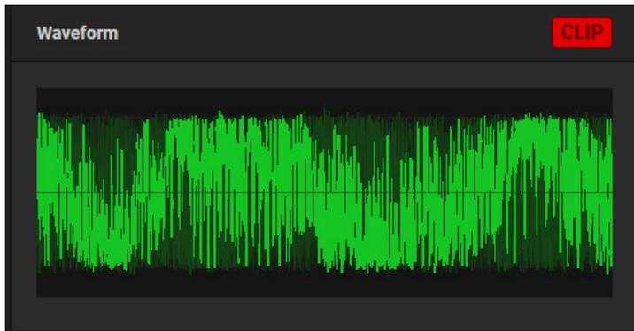
The Waveform display gives you a quick view of your audio levels, including a clip indicator that flashes when triggered by high levels. Input levels may be adjusted in the setup screen.
