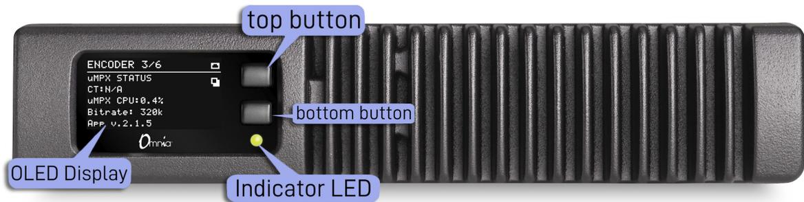
The MPX Node front panel consists of two buttons, an LED and a long-life OLED display, housed in a fanless, rugged cast aluminum body with integrated heat exchanger. The front panel provides fast access to system status information. Front panel data input is limited to IP address setup and password reset so you can get at the GUI, the real control point for all system operation.
