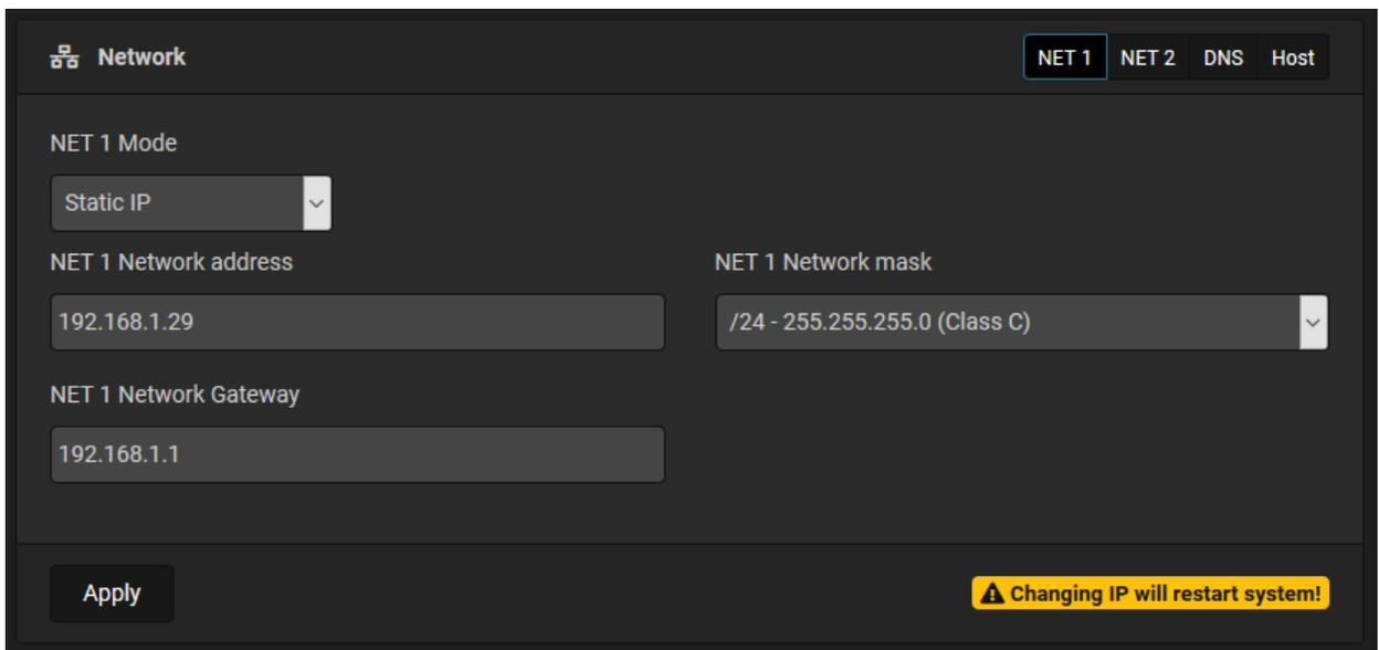
The screenshot shows the 'Network' configuration screen. At the top, there are tabs for 'NET 1', 'NET 2', 'DNS', and 'Host'. The 'NET 1' tab is selected. Below the tabs, the 'NET 1 Mode' is set to 'Static IP'. The 'NET 1 Network address' is '192.168.1.29' and the 'NET 1 Network mask' is '/24 - 255.255.255.0 (Class C)'. The 'NET 1 Network Gateway' is '192.168.1.1'. At the bottom left is an 'Apply' button, and at the bottom right is a warning icon with the text 'Changing IP will restart system!'.
