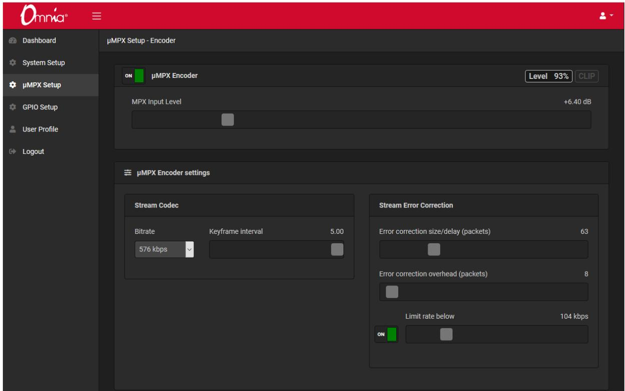
MPX Node Encoders come standard with 2 output streams. Traffic can be sent via Unicast, or Multicast to destination decoders. There are multiple use cases for stream output, for example:
