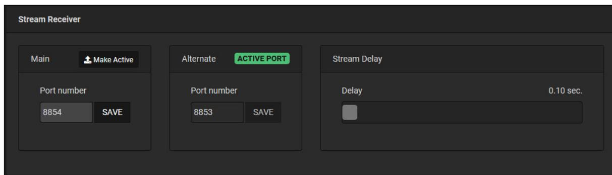
Port numbers can only be changed when a port is inactive, or the decoder is in the off position. Clicking on the “Make Active” button will switch ports, and a confirmation screen will display in the upper right corner.
