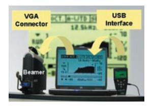
Distortion analyzer of the ML1. The small value (LVL) shows the level of the signal. The result of a broken cable is show in the above screen, indicated by the balance indicator (UBAL).
