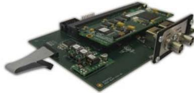
**This expansion board allows the monitoring of embedded audio channels within a single link 3G/HD/SD-SDI video signal. The embedded audio can be either non-encoded linear PCM, Dolby® E or Dolby® Digital. Please note that the RM-HDE1 card is for use with the RM-4C8 unit only.**
