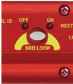
Fig 1-6: Sequence Loop Button & LEDs
